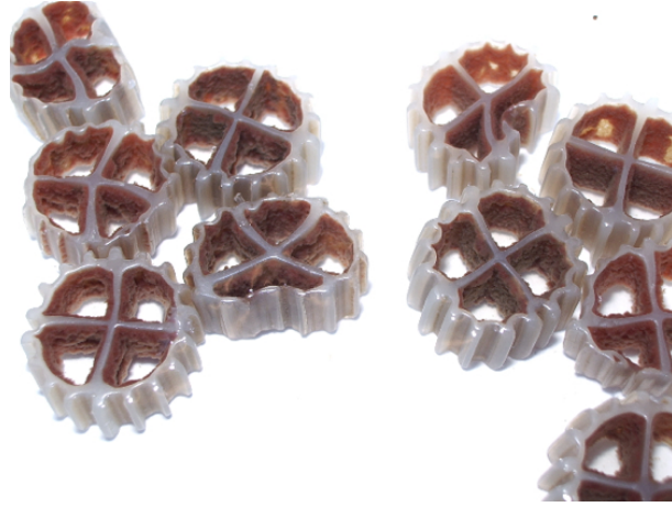
Figure 2.1: Carrier with anammox bacteria. Image source: The CONAN project
