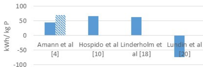
Fig. 2. Results for scenario 2 – use of fertilizer in agriculture produced from P extracted from ashes after drying and mono-incineration of sludge. For Amann et al. [4] the filled column represents the case with the lowest energy demand and the dashed column represents the highest energy demand.
